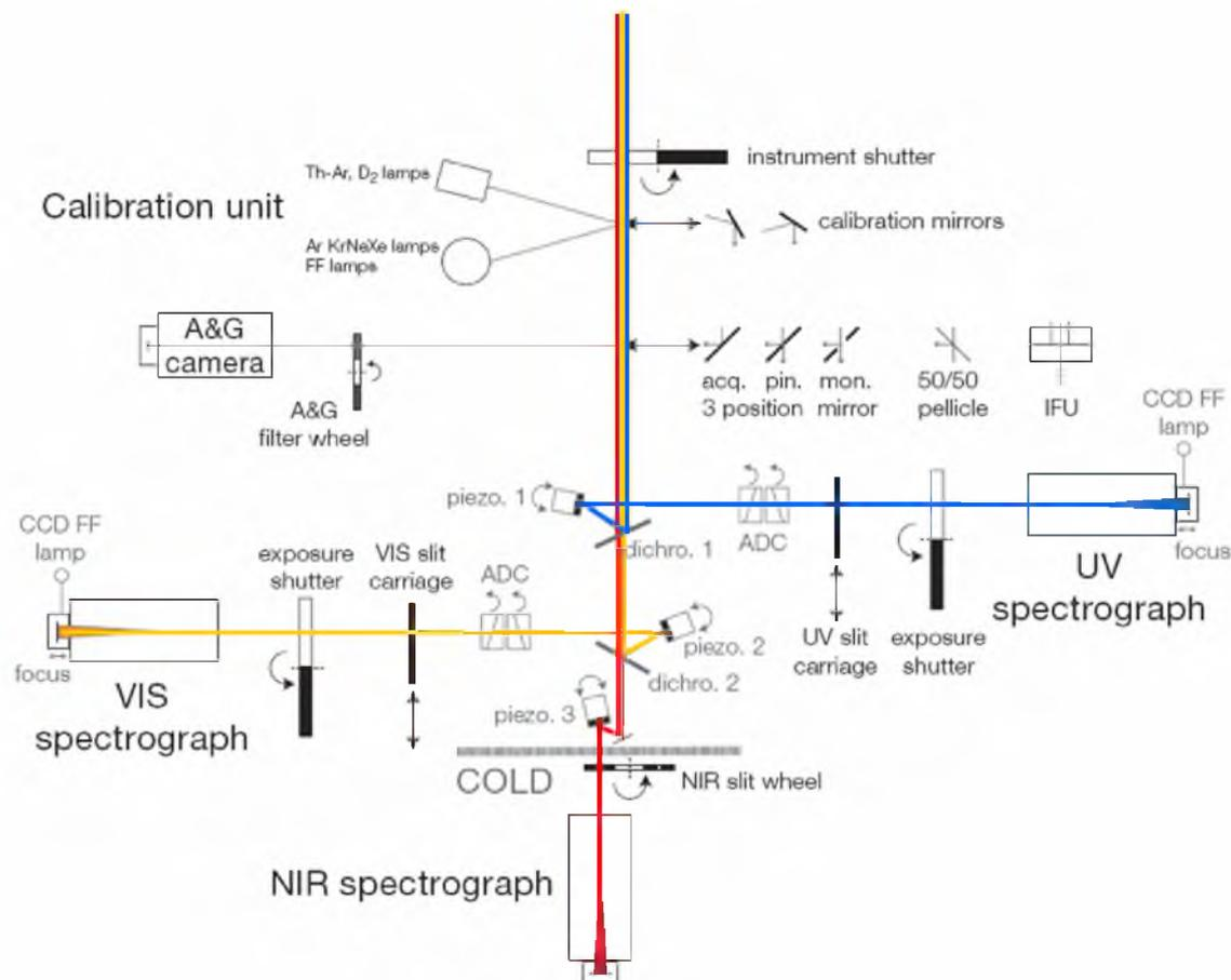
Figure 1. Schematic view of X-shooter
