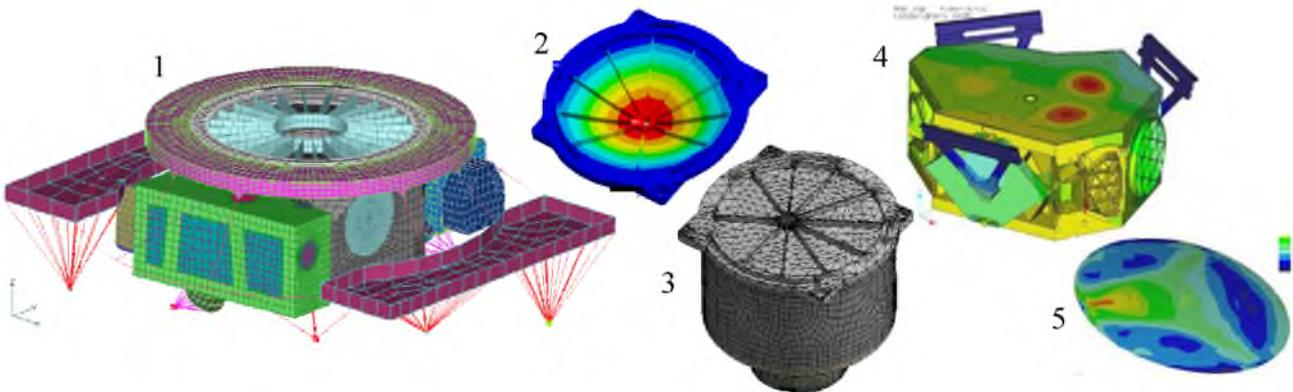
Figure 19. To predict instrument flexure behavior an extensive FEM analysis was performed during the design phase, consisting of 5 separate FEM models: The backbone<sup>1</sup>, the NIR cryostat deformation due to air pressure<sup>2</sup> and gravity<sup>3</sup>, the cold optics box<sup>4</sup> and individual mirrors<sup>5</sup>. The gravity direction is simulated at zenith and 12 rotation angles at 60° zenith distance.
