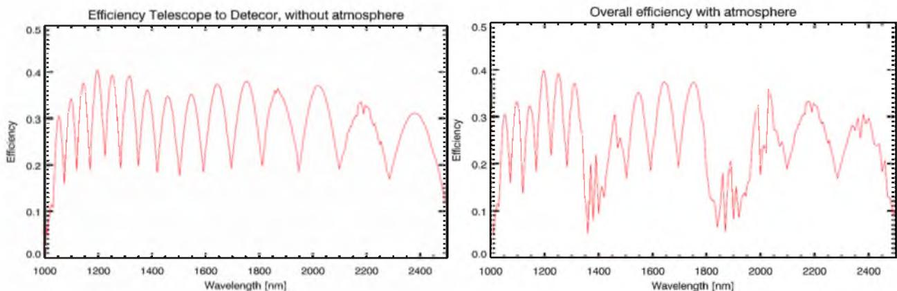
Figure 17. Efficiency of the X-shooter NIR spectrograph including efficiency of the Telescope, dichroics in the backbone and detector quantum efficiency. The efficiency is calculated from efficiencies of individual optical components and is shown without and with atmosphere transmission.
