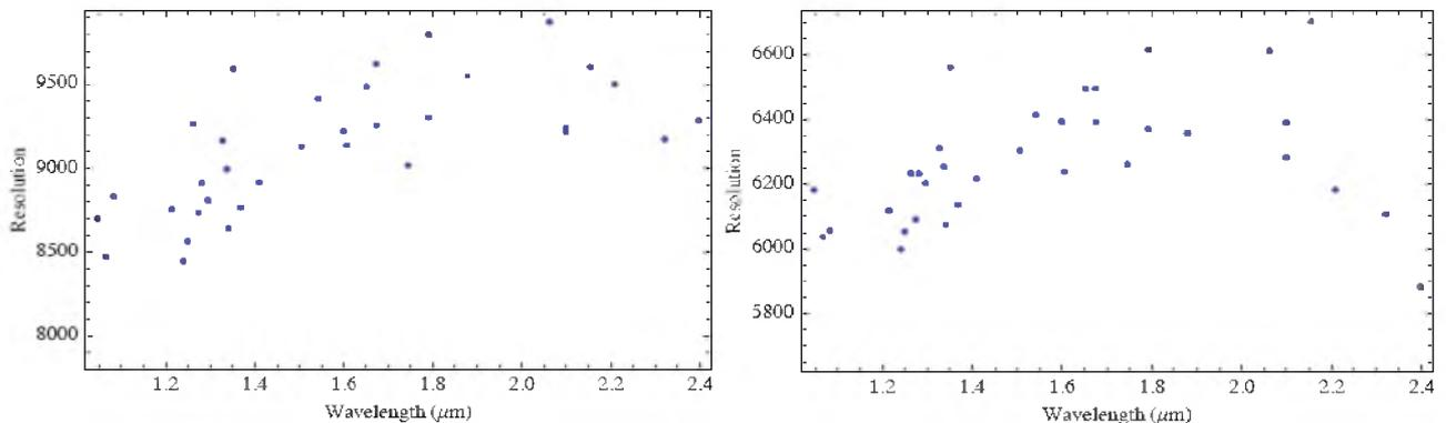
Figure 16. Spectral resolution measured with slit width of 0.6 arcsecond (left) and 1.0 arcsecond (right).
