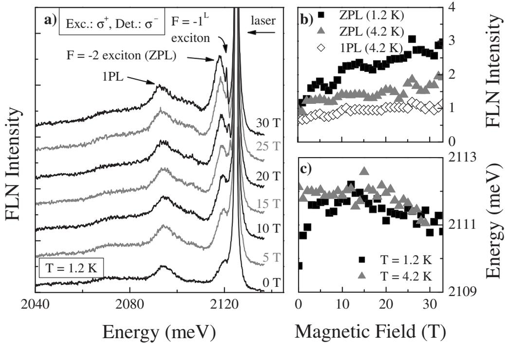
FIG. 3. (a) FLN spectra of QD2 with increasing magnetic field at 1.2 K with  $\sigma^+$  polarized excitation and  $\sigma^-$  detection. (b) The intensity of the ZPL emission at 1.2 (squares) and 4.2 K (triangles), and the 1PL intensity at 4.2 K (open diamonds) as a function of magnetic field. (c) The intensity weighted average energy position as a function of magnetic field at 1.2 K (4.2 K), squares (triangles).
