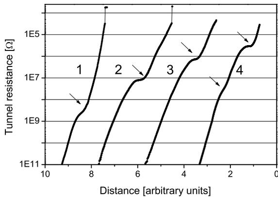
**Figure 1.** Distance tunneling spectroscopy of the physically adsorbed hydrogen molecules on the surface of Ta. In the course of time  $\text{H}_2$  tends to move towards the surface. Curve 4 displays the presence of a second layer of hydrogen molecules.
