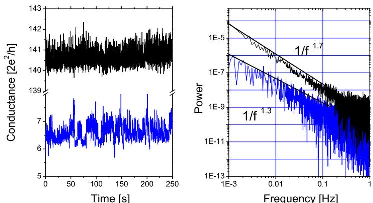
**Figure 4.** Typical pattern of conductance fluctuations for  $TaH_x$  junctions for  $G = 6.5 G_0$  and  $G = 140.5 G_0$ . The noise power spectra for the same junctions display  $1/f^\alpha$  law at  $f \leq 1 Hz$  with  $\alpha = 1.3$  and  $1.7$  respectively. In all cases  $V_b = 10 mV$ .
