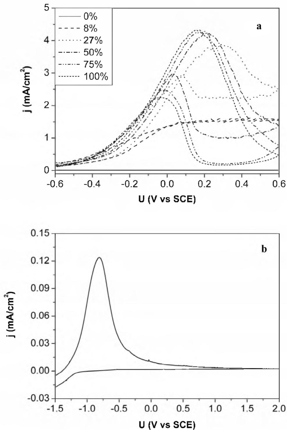
Figure 3. Current density-potential plots recorded for n-type 4H SiC at different light intensities (a) and n-type Si in the dark (b) in 0.1M KOH solution at 20.5 °C.
