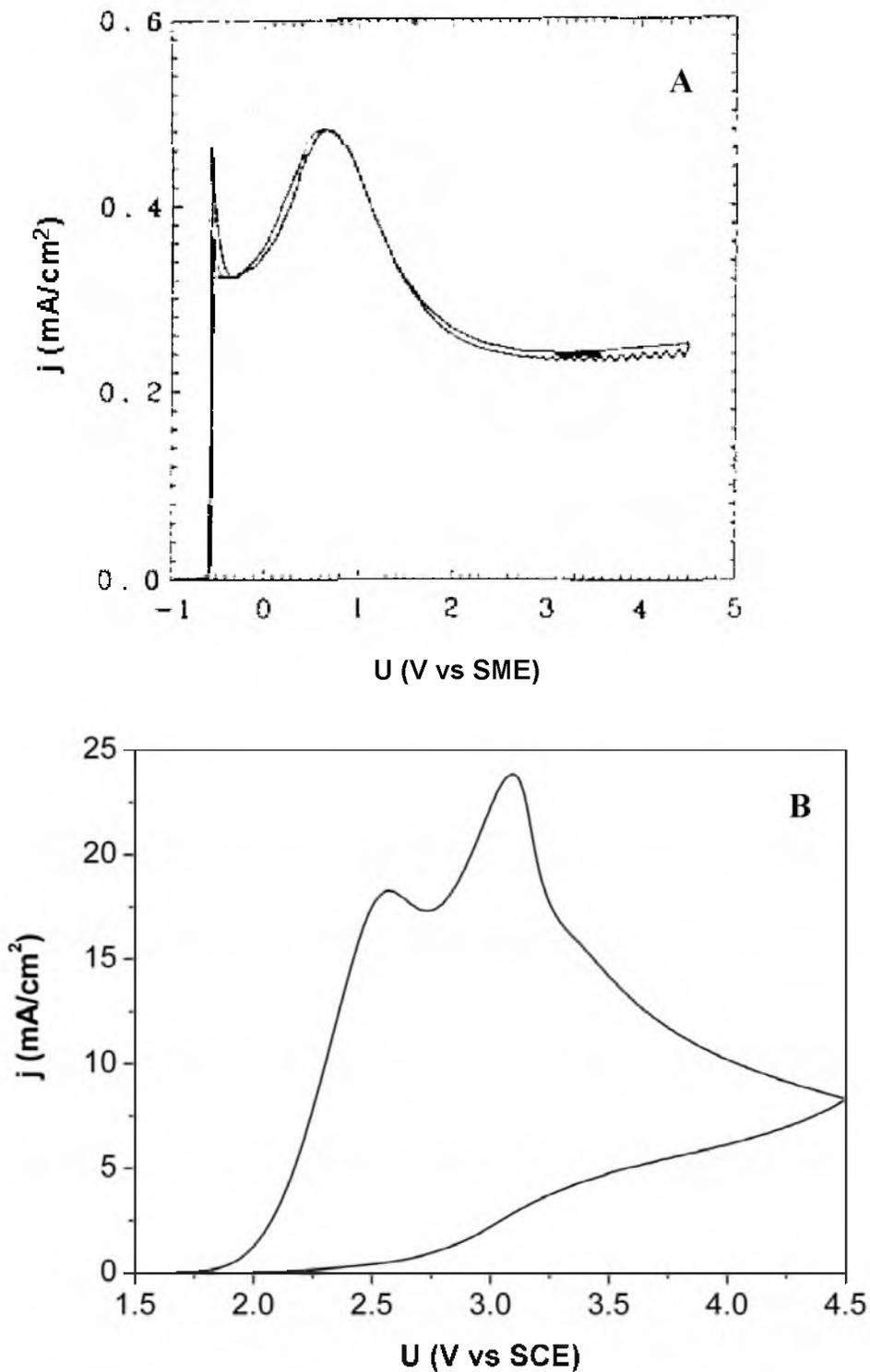
Figure 6. Current density-potential plots recorded in fluoride media ( $c_f = 33\text{mM}$ ,  $\text{pH}=3$ ) for p-type Si [21](a) and p-type 4H SiC (b). The rotation rates used were 1600 RPM and 1500 RPM for Si and SiC respectively. Note: In fig 6(a) the potential is given with respect to a saturated mercury/mercurous sulfate (SME) reference electrode.
