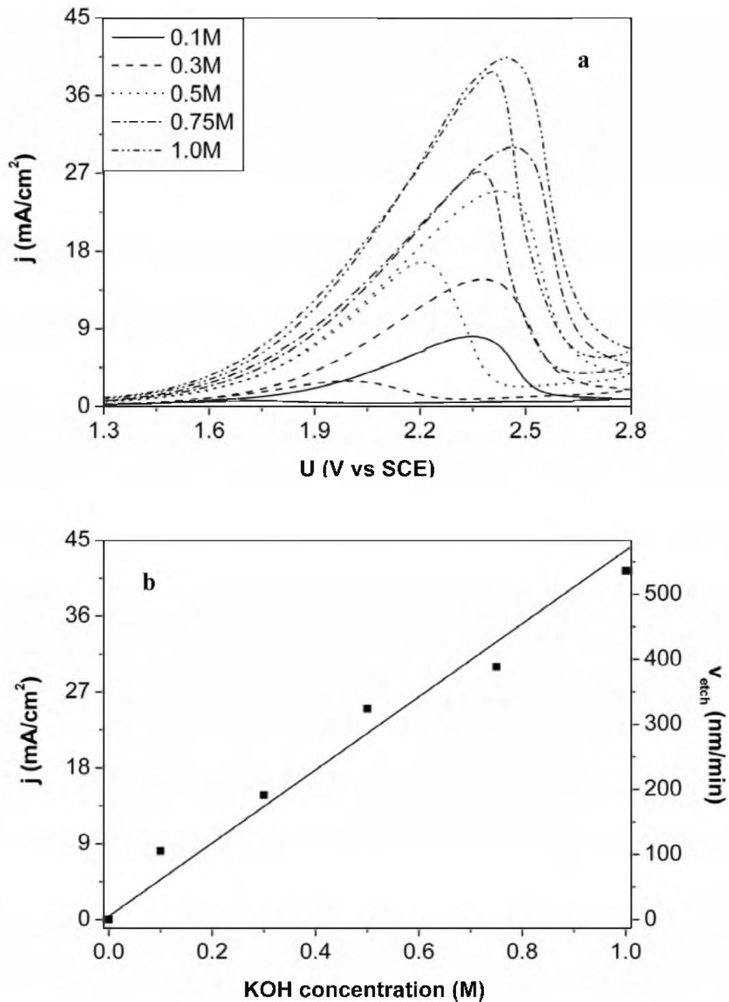
Figure 2. Current-potential curves for p-type 4H-SiC at different KOH concentrations at 20.5 °C (a). The values of the peak current and the passivation current are plotted against the KOH concentration (b). The right axis shows the calculated etch rate.
