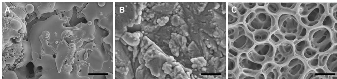
**Fig. 3.** Scanning electron micrographs of CaP coating morphologies of **A** plasma-spray coating, **B** RF magnetron sputter coating, and **C** electro spray deposition coating (*bar* represents 10  $\mu\text{m}$ ).
