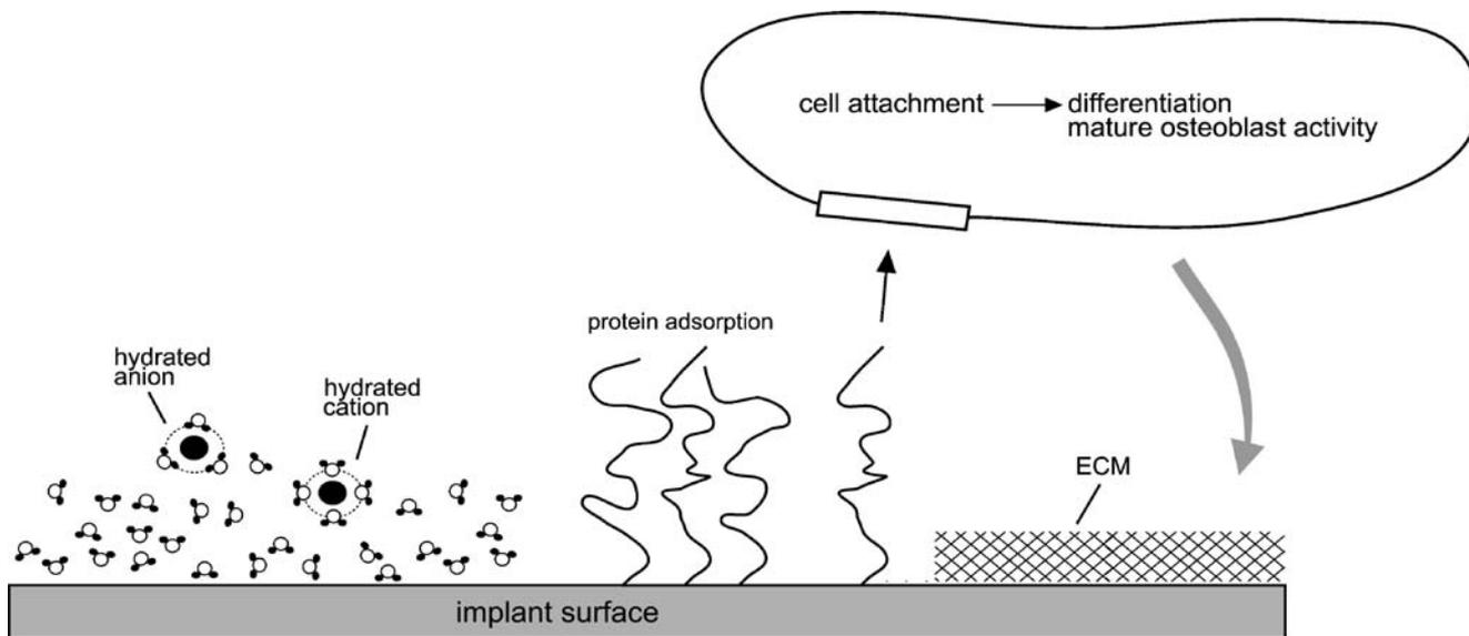
**Fig. 1.** Schematic representation of events consecutively taking place at the titanium surface after implantation into living bone tissue. Water binds to the surface, followed by incorporation of hydrated ions, adsorption and desorption of proteins, eventually leading to cell attachment. After differentiation, mature osteoblasts produce the extracellular matrix (ECM).
