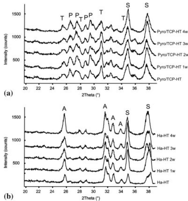
**Figure 4.** XRD patterns of sputtered Ca-P coatings after incubation in SBF; (a) pyro/TCP coatings (b) HA coatings.
