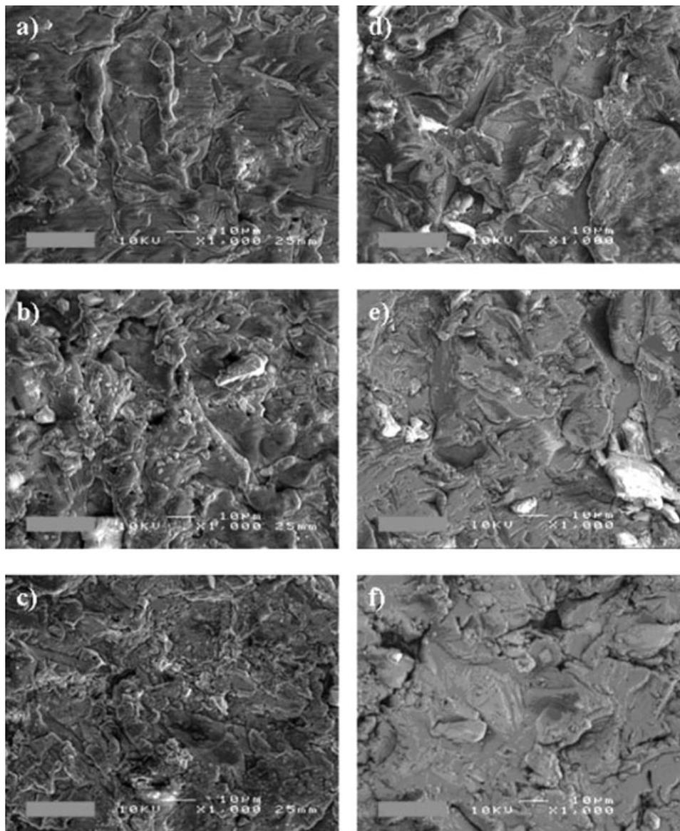
**Figure 3.** SEM pictures of coatings as-sputtered, heat-treated, and after incubation in SBF. (a–c) Pyro/TCP as-sputtered, and after 2 and 4 weeks SBF immersion; (d–f) HA as-sputtered, and after 2 and 4 weeks SBF immersion (Original magnification ×1000).
