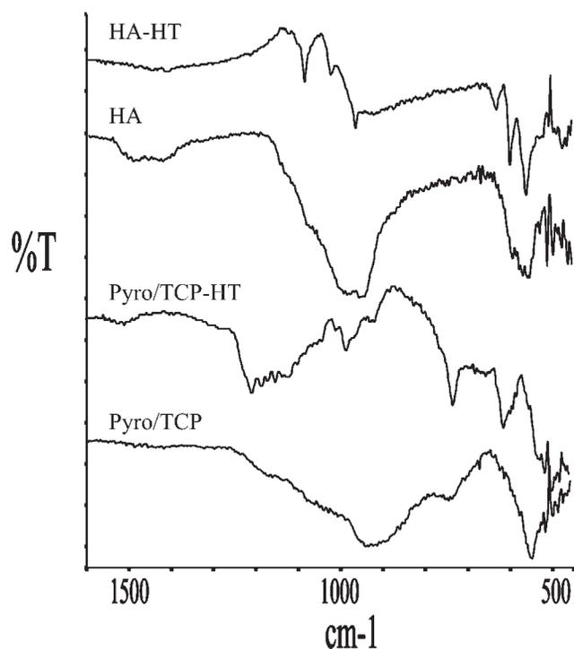
**Figure 2.** FTIR spectra of sputtered Ca-P coatings.
