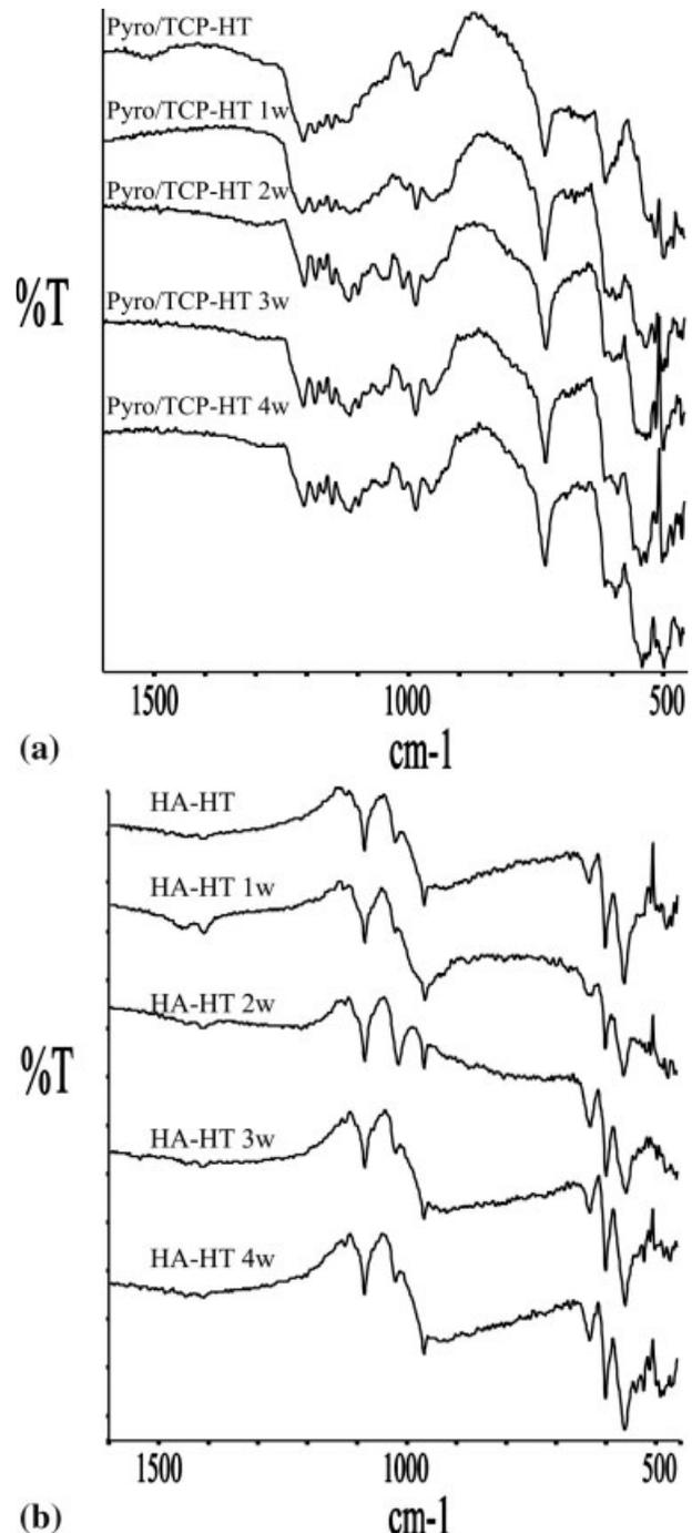
**Figure 5.** FTIR spectra of sputtered Ca-P coatings after incubation in SBF; (a) pyro/TCP coatings (b) HA coatings.
