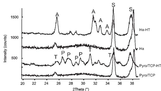
**Figure 1.** XRD patterns of sputtered Ca-P coatings. The major peaks have been marked: A, apatite; P, pyrophosphate; T, tri-calciumphosphate; S, substrate (titanium).
