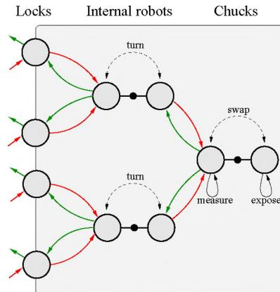
Fig. 1: Wafer paths within the EUV machine.
