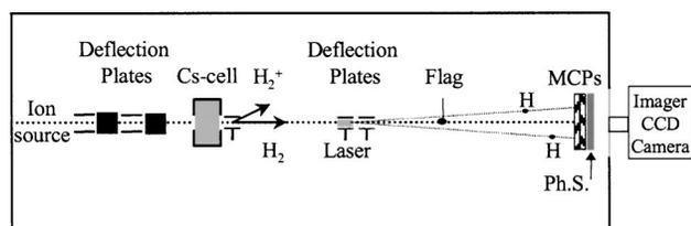
FIG. 2. Schematics of the apparatus. The molecular ion beam is produced in a hollow cathode ion source. The beam is extracted at 5 keV and neutralized via charge-transfer reactions with Cs. A pulsed laser beam crosses at 90° the neutral molecular beam. Once the photon is absorbed, predissociation and autoionization are the dominant decay paths of these high Rydberg states. A three-dimensional detector records the position ( $x, y$ ) and the arrival time  $t$  of each detected particle.
