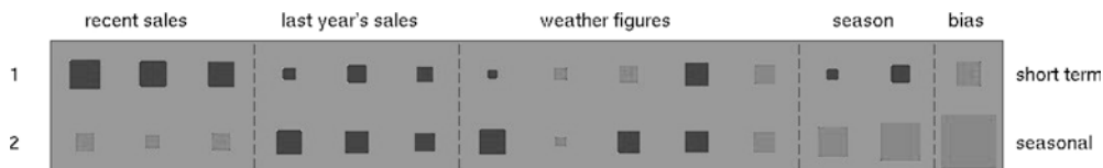
Fig. 3 A Hinton diagram of the hidden-to-input weights B_{jk} . Positive weights are white, negative weights are black. The absolute magnitude of each weight corresponds to the size of its square. Past sales figures are coded in inputs 1–6, inputs 7–11 represent weather information and 12–13 indicate the season. The rightmost squares represent the biases B_{j0} of the hidden units
