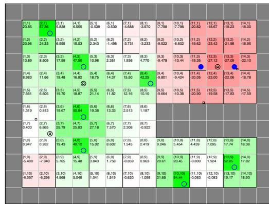
**Figure 1.** A grid environment with various walls. Potentials are visualized by color and denoted in each cell, below the cell’s coordinate. Gray cells lie outside the environment. Robots are visualized using circles (outlined for idle robots, filled for robots that are going to a resource). Resources are visualized using small black boxes. It can be seen that some resources are currently held by a robot (e.g., at (4,4)).
