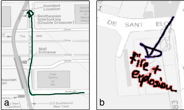
Figure 1. Two examples where context information can be of use in gesture recognition. (a) An arrow used to specify a route. (b) An arrow used to mark a location. The arrow in (a) follows the street pattern, the arrow in (b) does not.
