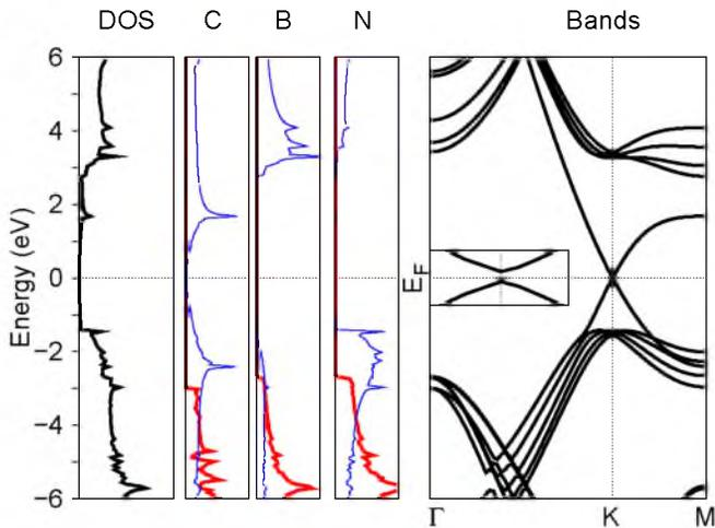
FIG. 3: (Color online) Band structure along the  $\Gamma K$  and  $KM$  directions in reciprocal space, total and projected densities of states (DOS) for the relaxed structure (c) of graphene on h-BN. Carbon, Boron and Nitrogen projected DOS are shown, with a projection on the  $p$ -states in-plane (red/thick grey lines) and out-of-plane (blue/thin grey lines). The inset is a magnification of the bands around the  $K$  point, where the gap opens.
