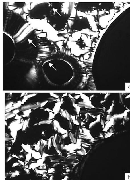
Figure 1. Defect textures of the smectic A phase of 6,6'-di-O-octanoylsucrose, **2a**, (x100); a) the oily streak texture and fanlike defects around air bubbles, b) the focal-conic defect and homeotropic textures.
