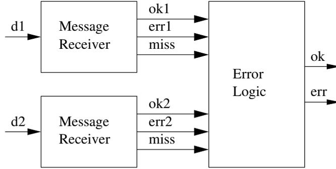
Figure 3: Decomposed architecture for two data sources
