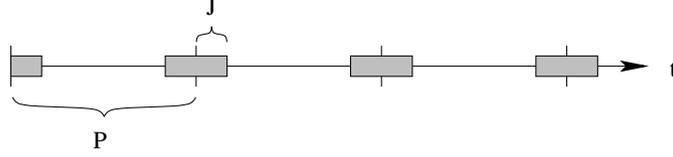
Figure 2: Data with period  $P$  and jitter  $J$
