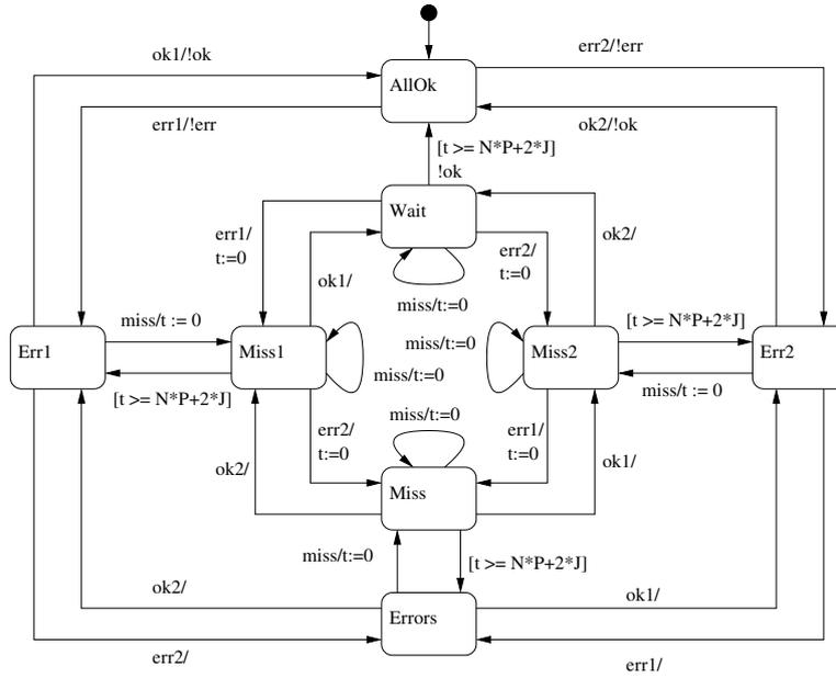
Figure 4: State Machine of the error logic component
