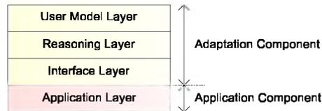
Figure 7. Layering of a user adaptive system
