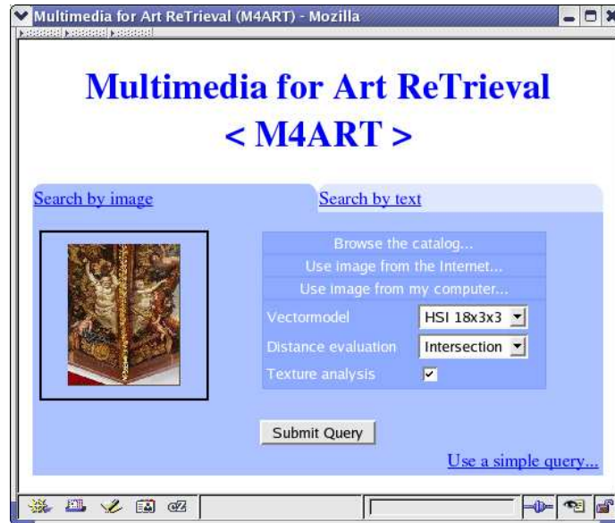
Figure 4. The advanced Content-Based Image Retrieval (CBIR) interface of the online Multimedia for Art ReTrieval (M4ART) system. An image can be selected through browsing the database, providing the URL of an image, or by uploading an image from the local hard-disk. A color space and its quantization scheme can be chosen; i.e., HSI 18 \times 3 \times 3 , 11 color categories, RGB 4 \times 4 \times 4 , or HSI 9 \times 6 \times 6 (see Section 3.2.1). A choice can be made between the intersection and Euclidean distance measure (see Section 3.3). Texture features can be selected to be taken in the processing scheme (see Section 3.2.2). The M4ART system is available at http://cai.nici.ru.nl/M4ART/ .
