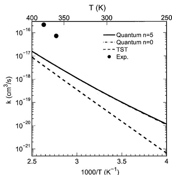
FIG. 1. Rate constants for the D+CH<sub>4</sub>→CH<sub>3</sub>+HD reaction.  $n$  is the number of vibrationally excited states of the activated complex included explicitly in the accurate quantum calculations [see Eq. (2)]. Experimental rate constants are taken from Ref. 25.
