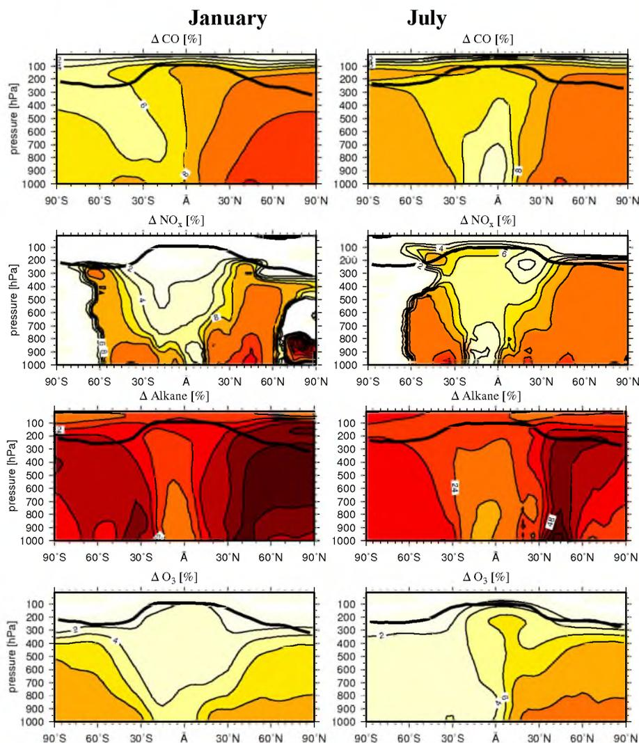
**Fig. 4.** Relative contribution of road traffic emissions to atmospheric CO, NO<sub>x</sub>, NMHCs and O<sub>3</sub> zonally averaged distributions (in %). Isolines are 2, 4, 6, 8, 12, 24, 32, 48, 56%.
