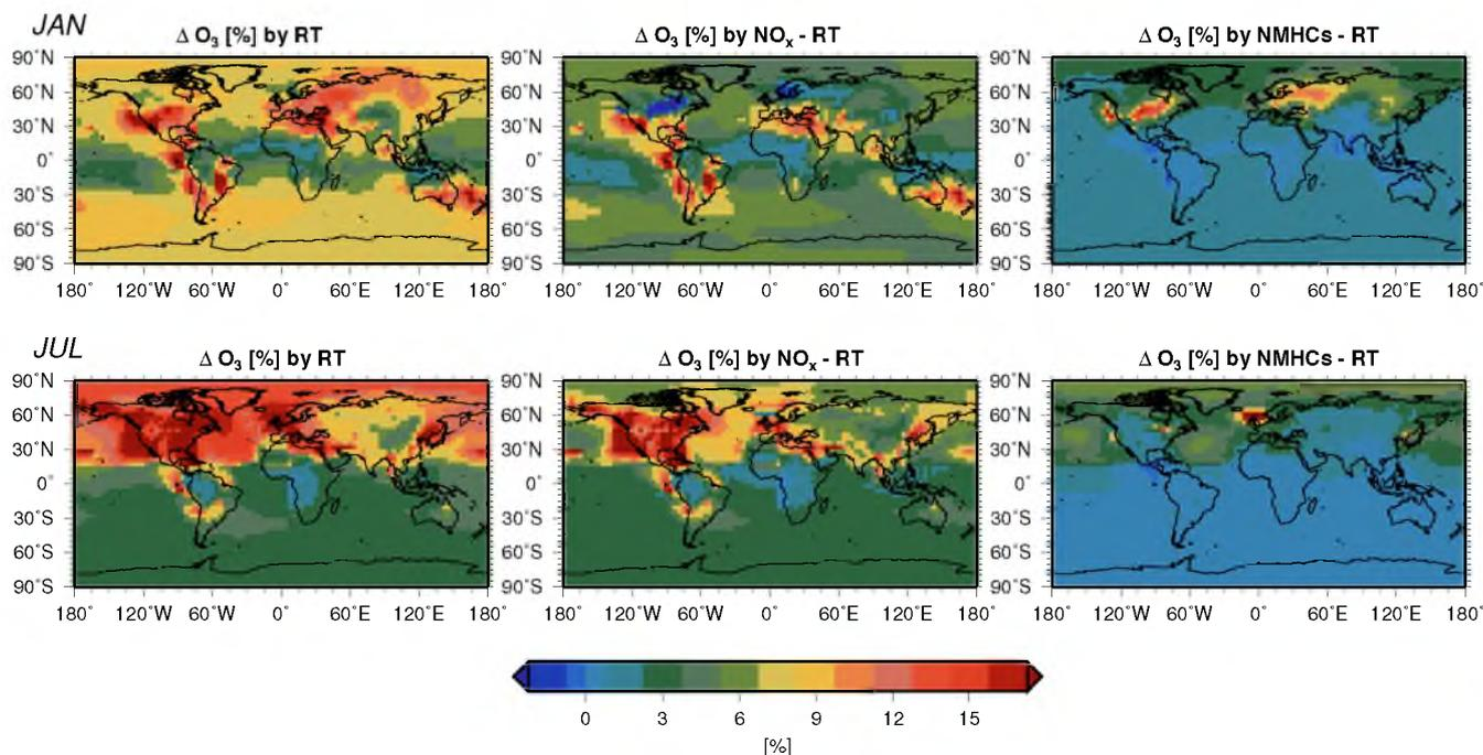
**Fig. 5.** Relative contributions [%] of total and individual road traffic emissions to the surface ozone distribution in January (upper row) and July (lower row); total emissions (left), NO<sub>x</sub> only (middle) and NMHC only (right).
