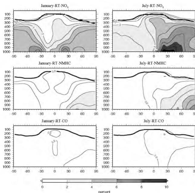
**Fig. 7.** Contributions [%] of individual road traffic emissions –  $\text{NO}_x$  (upper), NMHCs (middle) and CO (lower) to atmospheric distribution of ozone. Isolines are equidistant with 1% difference, plus one additional line for 0.5%.
