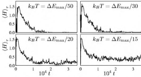
FIG. 6. Order parameter for collective motion  $\langle H \rangle_\tau$  as a function of time for different temperatures, and for  $\tau = \Delta t$ ,  $k_2 = 1$ ,  $\gamma = 0.5$ , and  $N = 10\,000$ . The solitary state is stable at least up to  $k_B T = \Delta E_{\max}/30$ .
