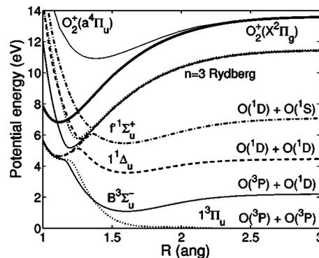
FIG. 1. Schematic of the potential curves relevant for the DR process with  $O_2^+$ . The electronic ground state  $X^2\Pi_g$  and the first ionic metastable state  $a^4\Pi_u$  are given. A number of neutral capture states is given in an adiabatic representation showing the consequences of the interaction with the  $n=3$  Rydberg states. The dissociation limits relevant for this work are given on the right hand side.
