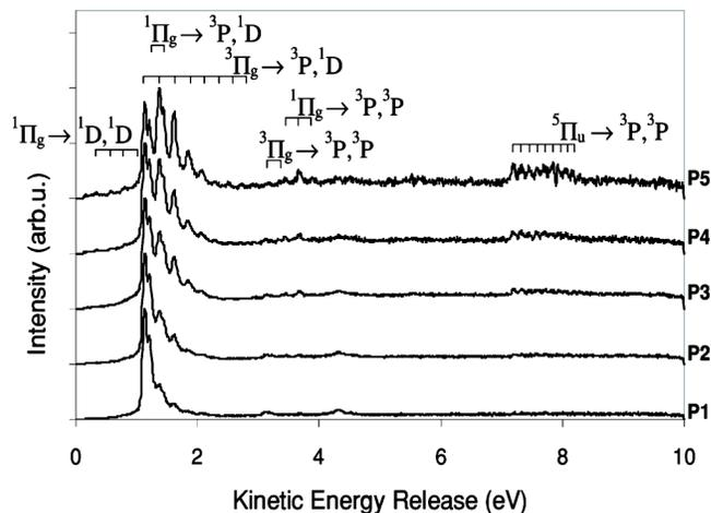
FIG. 4. Measured spectra from the Cs- $O_2^+$  DCT reaction for the five different ion-source settings (equivalently the five vibrational populations), P1–P5.
