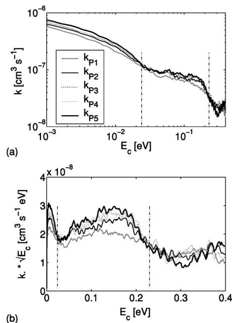
FIG. 5. (a) The total rate coefficients,  $k_{P_i}$ , as function of collision energy,  $E_c$ , up to 0.4 eV where  $P_i=P1-P5$ , on a bi-logarithmic scale, (b) and on a bilinear scale when multiplied by the square root of the collision energy, revealing the resonances due to nondirect dissociation mechanisms. The dashed vertical lines at 0.024 and 0.23 eV indicate the energy of the spin-orbit splitting in the  $X^2\Pi_g$ , ( $\Omega=1/2,3/2$ ) states and the vibrational spacing, respectively.
