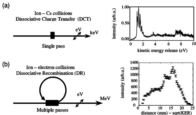
FIG. 2. Schematic diagram of (a) the dissociative charge transfer (DCT) experiment used to characterize the five vibrational populations of  $O_2^+$  used in the DR experiment shown in (b).
