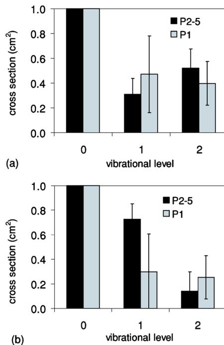
FIG. 7. The partial cross sections,  $\sigma_v$ , for  $v=0-2$ , relative to  $\sigma_0$ , at 0 eV collision energy resulting from the simultaneous fit of P2–P5 data (black) and the separate fit of P1 data (gray) obtained during storage times (a) 2.5–4.0 s and (b) 5.5–7.0 s.
