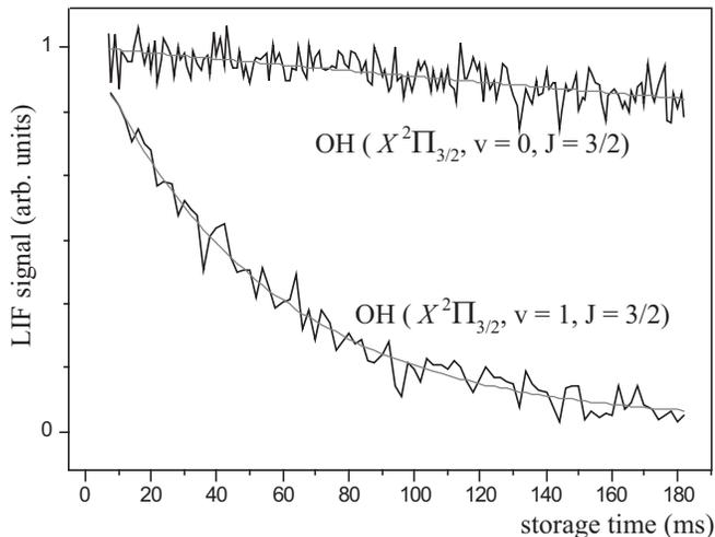
FIG. 2: Population of trapped OH radicals in the  $X^2\Pi_{3/2}, v = 0, J = 3/2$  level (upper curve) and in the  $X^2\Pi_{3/2}, v = 1, J = 3/2$  level (lower curve), as a function of the storage time  $t$ . The trapping potential is switched on at  $t = 0$  ms.
