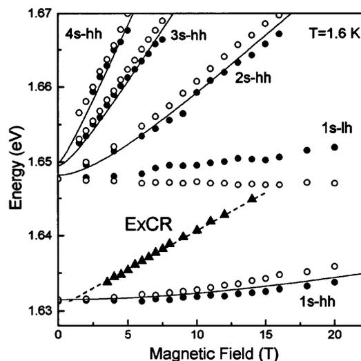
FIG. 3. Magnetoexciton fan chart of a 75 Å CdTe/Cd<sub>0.74</sub>Mg<sub>0.26</sub>Te QW. Closed and open symbols correspond to different spin orientations of the exciton states excited by  $\sigma^-$  and  $\sigma^+$  polarized light, respectively. The solid lines show the result of a calculation according to Ref. [9]. The new ExCR line is plotted by triangles with a dashed line as a guide for the eye (only the strong  $\sigma^-$  polarized component is shown).
