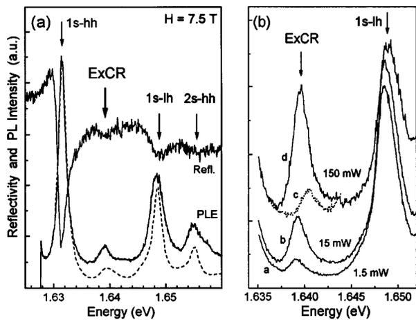
FIG. 2. (a) PLE and reflectivity spectra measure at a magnetic field of 7.5 T. The signal was detected on the X<sup>-</sup> line in  $\sigma^-$  circular polarization. The calculated absorption spectrum is shown by the dashed line. (b) PLE spectra taken under different intensities of the illumination (labeled in figure). Here, the PL is detected on the X line in  $\sigma^-$  polarization, with  $\sigma^-$  and  $\sigma^+$  polarized excitation for the solid and dotted lines, respectively.
