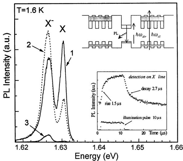
FIG. 1. Photoluminescence spectra of a 75 Å CdTe/Cd<sub>0.74</sub>Mg<sub>0.26</sub>Te QW taken under different excitation conditions: 1—direct excitation in the QW only, 2—direct excitation and illumination above the SL band gap, and 3—illumination only. The inset shows temporal changes of the X<sup>-</sup> line intensity measured under pulsed illumination (open circles).
