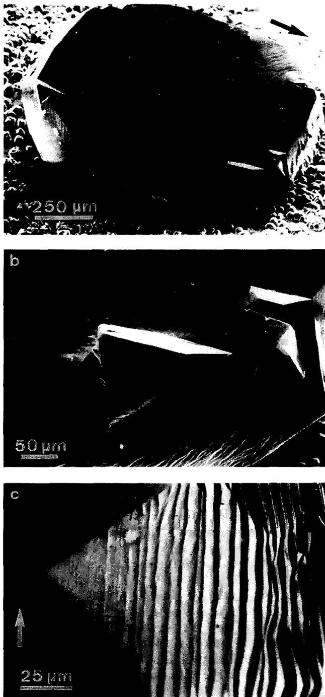
Fig. 2. Step sources on a {001} flame-deposited diamond film ( $T_{\text{dep}} = 1200^\circ\text{C}$ ,  $S_{\text{ac}} = 4\%$ ): (a) SEM image of surface morphology of a layer grown on a substrate with a misorientation of  $4^\circ$  towards {100}; (b) SEM image of detail of (a) showing a cusp on the edge with one of the {100} side faces; (c) DICM image of detail of (a) showing a large growth hillock on the top face. Arrows indicate  $\langle 110 \rangle$  directions.
