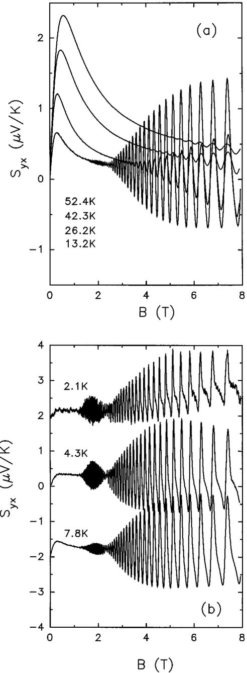
FIG. 5. Examples of the Nernst-Ettingshausen coefficient  $S_{yx}$  as a function of magnetic field. Data in panel (a) are at higher temperatures, and those in panel (b) at lower temperatures. In panel (b) the curves at 2.1 and 7.8 K have been offset by 2  $\mu\text{V}/\text{K}$ .
