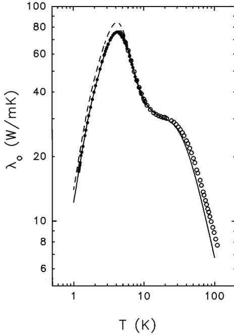
FIG. 2. The measured zero-field thermal conductivity  $\lambda_o$  as a function of temperature. The two sets of symbols correspond to two different cooldowns. The solid line is fitted using the model of Whitsett *et al.*, as described in the text, for the lattice thermal conductivity  $\lambda_o^g$ . The dashed line shows the effect of turning off the phonon-electron scattering in the calculation.
