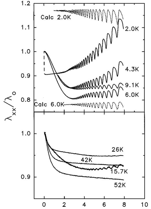
FIG. 3. The thermal conductivity  $\lambda_{xx}$  as a function of field at various temperatures. The data are normalized to the zero-field values  $\lambda_o$ . In the upper panel the dotted curves are calculations of the oscillations at 2 and 6 K assuming they are due to  $p$ - $e$  scattering.
