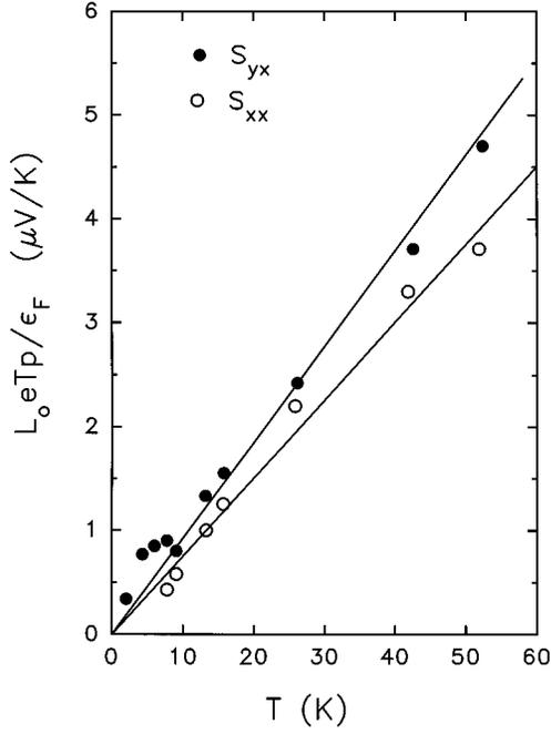
FIG. 6. The quantity  $L_0 e T p / \epsilon_F$  obtained from fits to the nonoscillatory parts of  $S_{yx}$  and  $S_{xx}$ , respectively, as a function of temperature.
