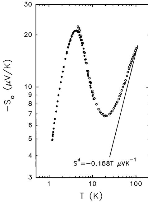
FIG. 4. The thermopower at zero field  $S_0$  as a function of temperature. The two sets of symbols are the same two cooldowns as mentioned in Fig. 1. The straight line is the estimated diffusion component.
