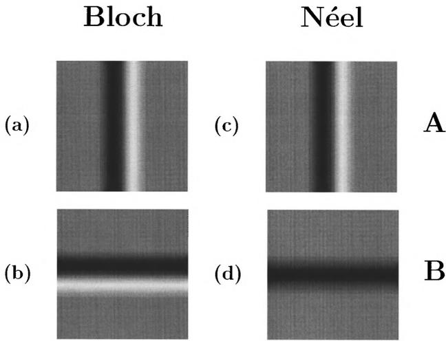
FIG. 4. Simulated images of fragments *A* (panels a, c) and *B* (b, d) of a Bloch (a, b) and Néel (c, d) wall in an odd-fold rotation symmetry film. The MSHG response is polarized along the vertical *y* azimuth. The fundamental field is assumed to be polarized purely along the *x* or *y* azimuth.
