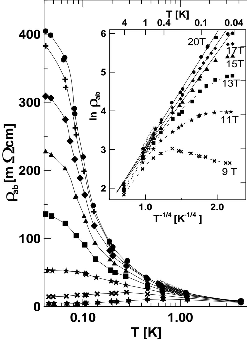
FIG. 2. The temperature dependence of  $\rho_{ab}$  for film S1 in perpendicular magnetic fields. The fields are, from below, 7, 9, 11, 13, 15, 17, 19, and 20 T. The open circles between  $T = 0.7$  K and  $T = 1$  K show the data obtained with dc as explained in the text. The lines are guides to the eye. The inset shows  $\ln \rho_{ab}$  versus  $T^{-1/4}$  for several magnetic fields.
