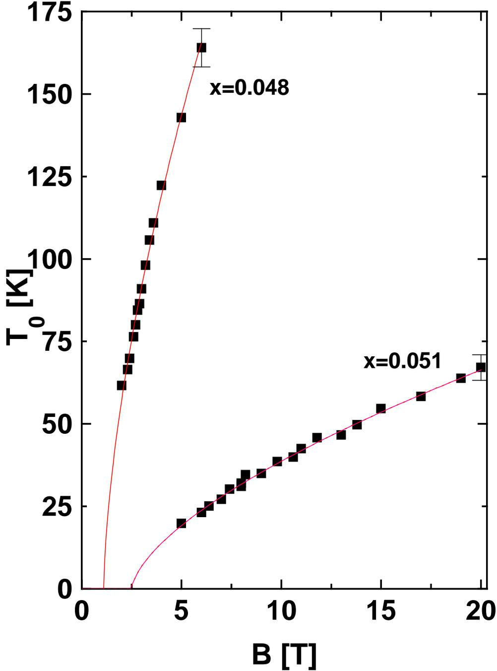
FIG. 5. The dependence of the parameter  $T_0$  on magnetic field for films S1 ( $x = 0.051$ ) and S2 ( $x = 0.048$ ). The error bars show the uncertainty resulting from the fit of the Mott relation to the data for the highest magnetic field. The dashed lines show the expression  $T_0 = A[(B - B_{cr})/B_{cr}]^\nu$ , fitted to the data, with the parameters  $A$ ,  $B_{cr}$ , and  $\nu$ , as described in the text.
