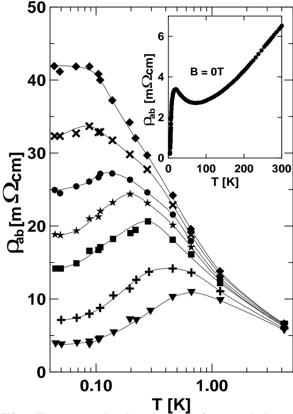
FIG. 1. The temperature dependence of  $\rho_{ab}$  for film S1 in perpendicular magnetic fields. The fields are, from below, 7, 8, 9, 9.4, 9.8, 10.2, 10.6 T. The open circles between  $T = 0.7$  K and  $T = 1$  K show the data obtained with dc as explained in the text. The lines are guides to the eye. The inset shows  $\rho_{ab}(T)$  in zero field.
