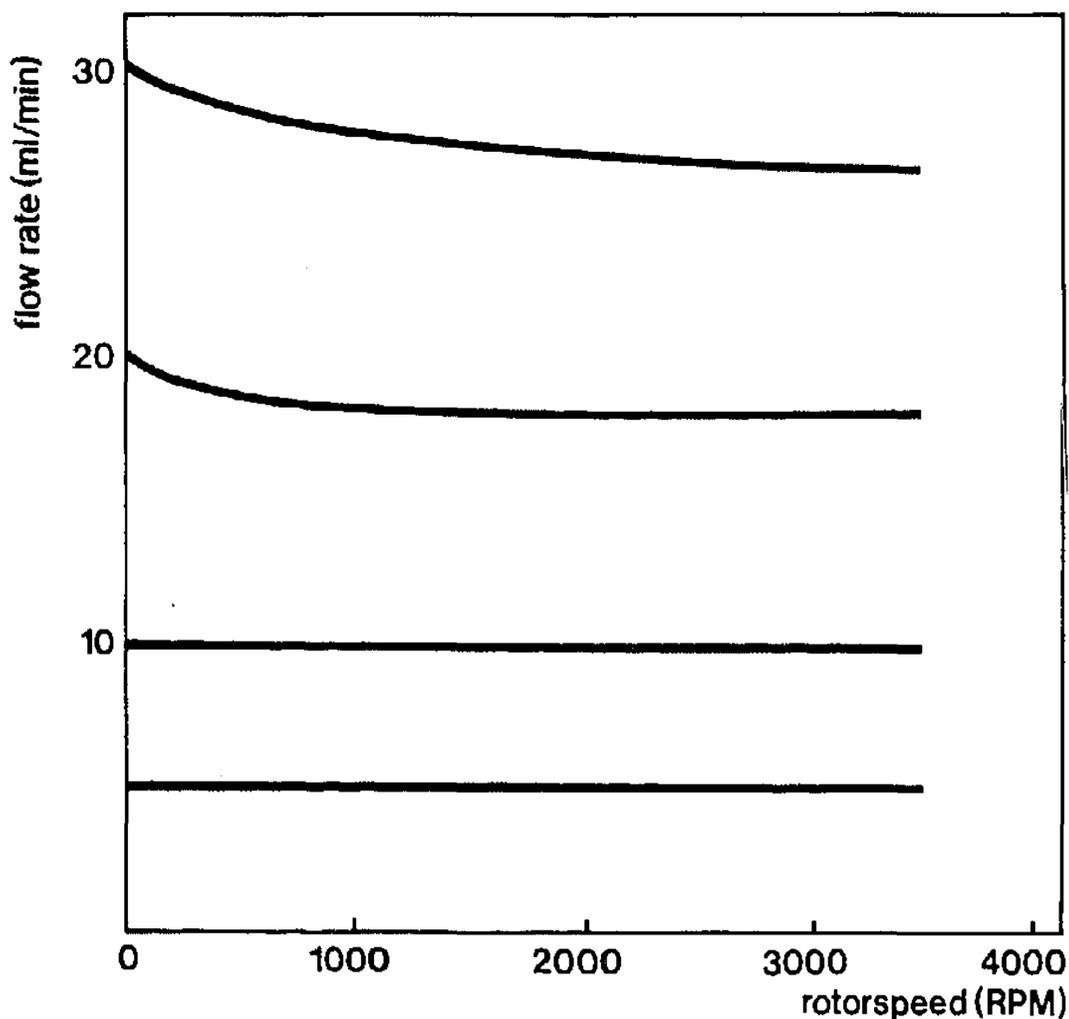
Fig. 3. Flow rate as a function of rotor speed. At a pressure of 180 cm the flow rate,  $F$ , was set at 4 values with clamp C (see Fig. 1). At each setting of the clamp the flow rate was measured as a function of rotor speed.
