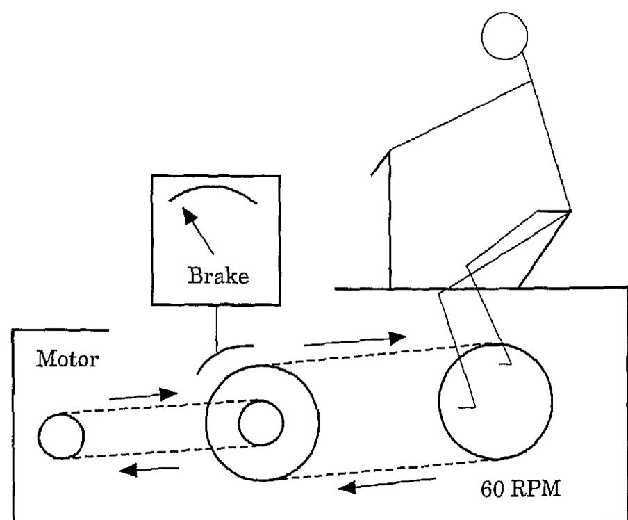
FIG. 1. Schematic presentation of a cycle ergometer for eccentric exercise. The pedals are driven in backward direction at a rate of 60 revolutions min<sup>-1</sup> (RPM) by the electric motor, which has to overcome the adjustable resistance of the electromagnetic brake. After withdrawal of the brake, the subject has to maintain a backward pedalling rate of 60 RPM by braking the speed of the pedals.
