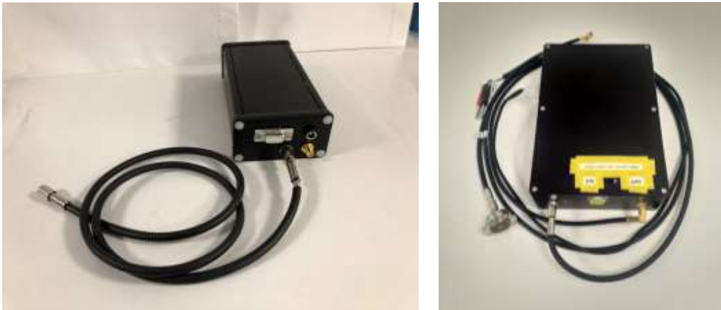
Figure 1. Left: Picture of the first miniature prototype, with dimension 80 \times 120 \times 46 \text{ mm}^3 and 5V power supply. Right: Picture of the final prototype, with dimension 220 \times 150 \times 55 \text{ mm}^3 and 24V power supply.
