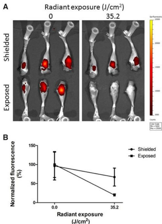
(A) Images of fluorescence observed at baseline and after  $35.2 \text{ J}/\text{cm}^2$  radiant exposure. (B) Quantification of mean fluorescent intensity normalized to baseline. Quantification of the fluorescent signal shows a faster decrease in the knee joints that were exposed to light when compared with the shielded group ( $P < 0.01$ ). Data are shown as mean (s.d.).  $n = 3$  mice/group.
