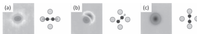
FIGURE 4.2 STM images and corresponding schematic representations of (a) bis-deuteroacetylene, (b) deuterioethynyl and (c) dicarbon. (Reprinted with permission from Lauhon et al., 2000. Phys. Rev. Lett. 84: 1527–30. Copyright (2000) by the American Physical Society.)
