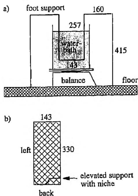
Side view of the foot volume recorder (a) and top view of the immersed bottom of foot support (b). Measures of foot support (in millimetres) are indicated by the numbers. The Perspex water bath measuring 388 mm × 208 mm × 250 mm had a maximal capacity of 20 l. The left foot of the subject is immersed within the water bath and placed on the bottom of the foot support with the heel against the niche in the back.
