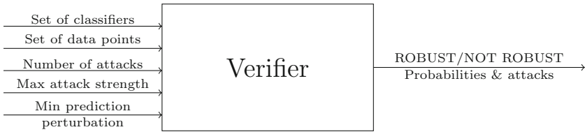
Fig. 2. The verifier takes as input a set of classifiers, a set of labelled data points, the number of attacks, and the attack properties. If the verifier does not find a solution, we can be sure is robust against any attack with the specific properties. Otherwise, it returns the optimal attack.
