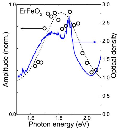
FIG. 3. Amplitude of the THz waveforms as a function of the pump photon energy (open circles) shown along with the measured optical density of the  $\text{ErFeO}_3$  sample (solid line). The amplitude is normalized as in Fig. 2. Dashed line is a guide to the eye. The narrow feature at  $\sim 1.87$  eV is due to  $f-f$  transitions in  $\text{Er}^{3+}$  ions. This measurement was performed at room temperature.
