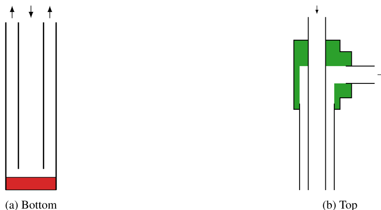
Fig. 4. Schematics of the concentric capillaries for stopped-flow experiments. At the bottom (a), the outer capillary is closed with glue (shown in red). At the top (b), a T-junction separates the inwards and outwards flow. (For interpretation of the references to colour in this figure legend, the reader is referred to the web version of this article.)
