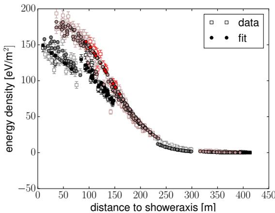
**Figure 1.** An example of a reconstructed air shower measured by LOFAR. The energy density is given as function of the distance to the shower axis. The colors indicate different azimuth angles. The red, pink, grey, and black points correspond to the northeast, southeast, southwest and northwest direction, respectively.
