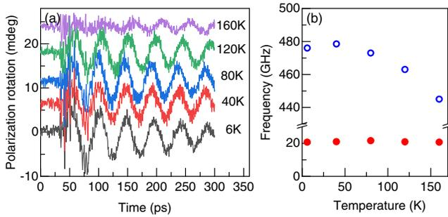
FIG. 4. (a) Optically detected THz induced spin dynamics at different temperatures, indicated near the curves. In the experiment the crystal was tilted around the  $y$  axis over  $10^\circ$ , as shown in Fig. 1(a).  $B_{\text{ext}} = 40$  mT. (b) Frequencies of the q-AFM (open blue circles) and q-FM (closed red circles) modes of the waveforms from panel (a).
