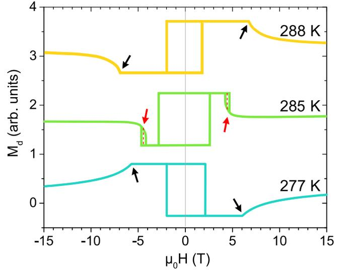
FIG. 3. Dependence of the component of the  $d$ -sublattice magnetization along the easy-axis direction on the magnetic field at different temperatures. Black and red arrows indicate second- and first-order transition points, respectively.
