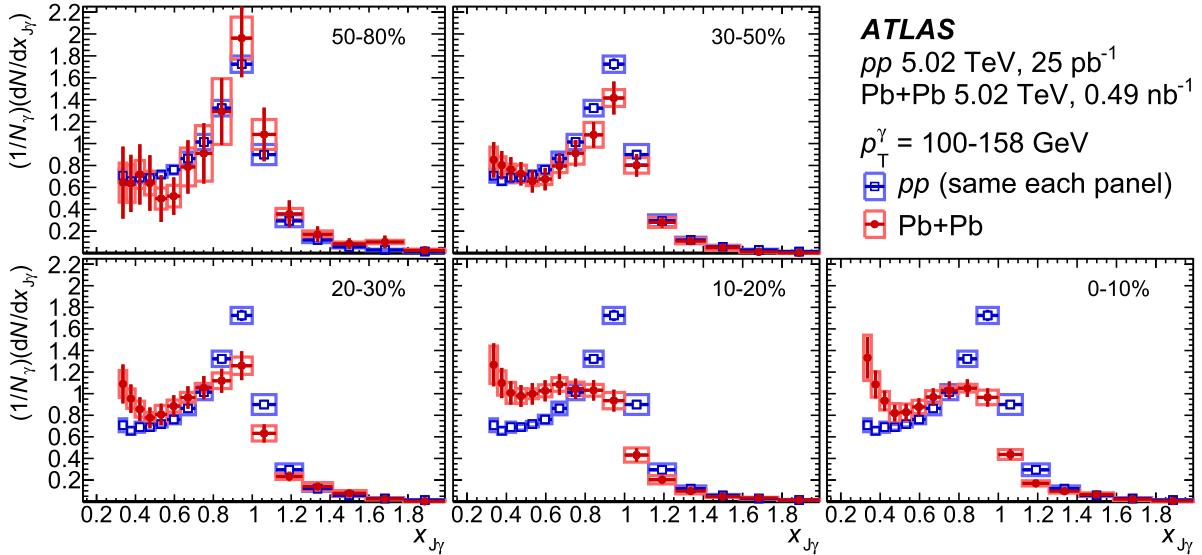
**Fig. 6.** Photon-jet  $p_T$ -balance distributions  $(1/N_\gamma)(dN/dx_{J\gamma})$  in  $Pb + Pb$  events (red circles) with each panel showing a different centrality selection compared to that in  $pp$  events (blue squares). These panels show results for  $p_T^\gamma = 100\text{--}158 \text{ GeV}$ . Total systematic uncertainties are shown as boxes, while statistical uncertainties are shown as vertical bars.
