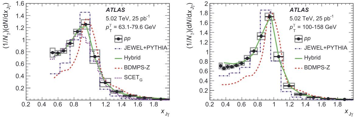
**Fig. 9.** Photon-jet  $p_T$ -balance distributions  $(1/N_\gamma)(dN/dx_{J\gamma})$  in  $pp$  collisions for (left)  $p_T^\gamma = 63.1\text{--}79.6 \text{ GeV}$  and (right)  $p_T^\gamma = 100\text{--}158 \text{ GeV}$ . The unfolded results are compared with the theoretical calculations shown as dashed coloured lines (see text). Total systematic uncertainties are shown as boxes, while statistical uncertainties are shown as vertical bars.
