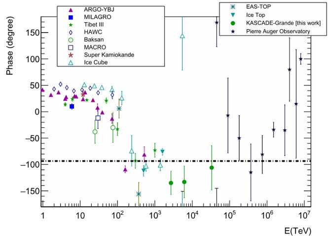
**Figure 6.** Comparison of the KASCADE-Grande measurements of the phase of the first harmonic with experimental results obtained in the energy range of  $10^{13} < E < 10^{19}$  eV. The dotted line shows the direction of the galactic center. The references to the results of the other experiments can be found in the caption of Figure 5.
