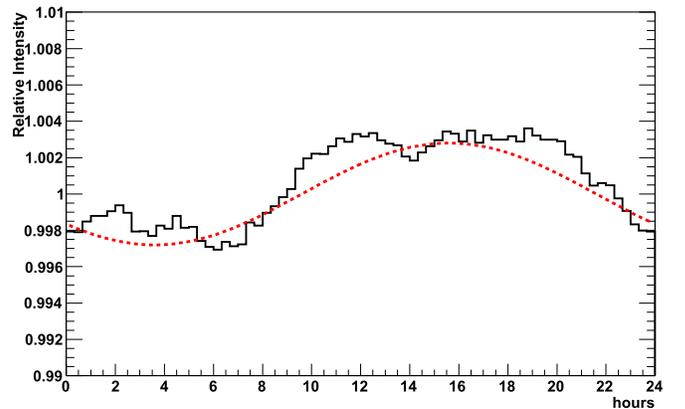
**Figure 3.** Sidereal time variations of the number of counts obtained, in 20 minutes intervals, by applying the east–west method. The dashed line represent the first harmonic fit; the amplitude and phase values are reported in Table 1.
