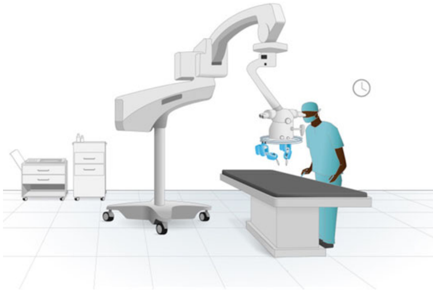
FIGURE 1 Schematic set-up of the MicroSure robot. The system can be attached to a surgical microscope or to the operation table [Color figure can be viewed at wileyonlinelibrary.com ]
