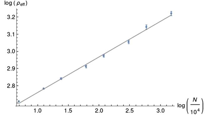
FIG. 7. Log-log plot of the effective radius  $\rho_{\text{eff}}$  as a function of the volume  $N$ , together with a linear fit, leading to  $\mathcal{D} = 4.85(16)$ . In the case shown,  $\rho_{\text{eff}}$  was extracted from fitting to a five-sphere (i.e.,  $D = 5$ ) and using an additive shift.
