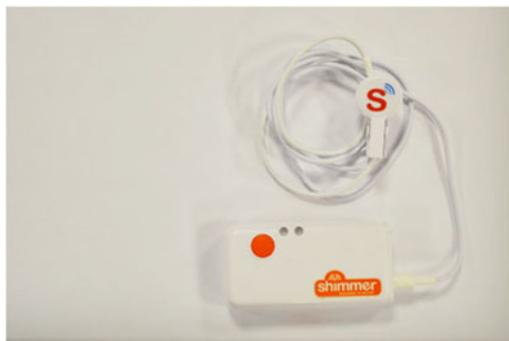
Fig. 5. Shimmer sensor with PPG ear clip.
