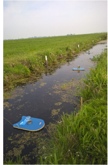
Diffusive flux measurements with floating chamber and Los Gatos (left) and bubble traps for ebullitive flux measurements (right)
