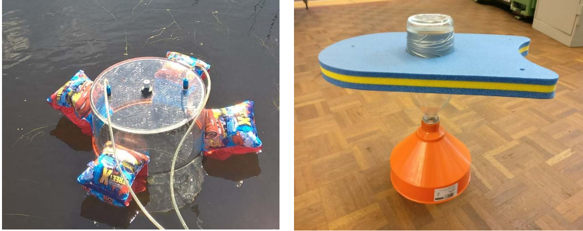
Figure 1: Floating chamber used to measure diffusive fluxes (left) and bubble traps used for ebullitive flux measurements (right). In ditches with low water levels (<30 cm) smaller bubble traps were used (smaller funnel and smaller bottle)
