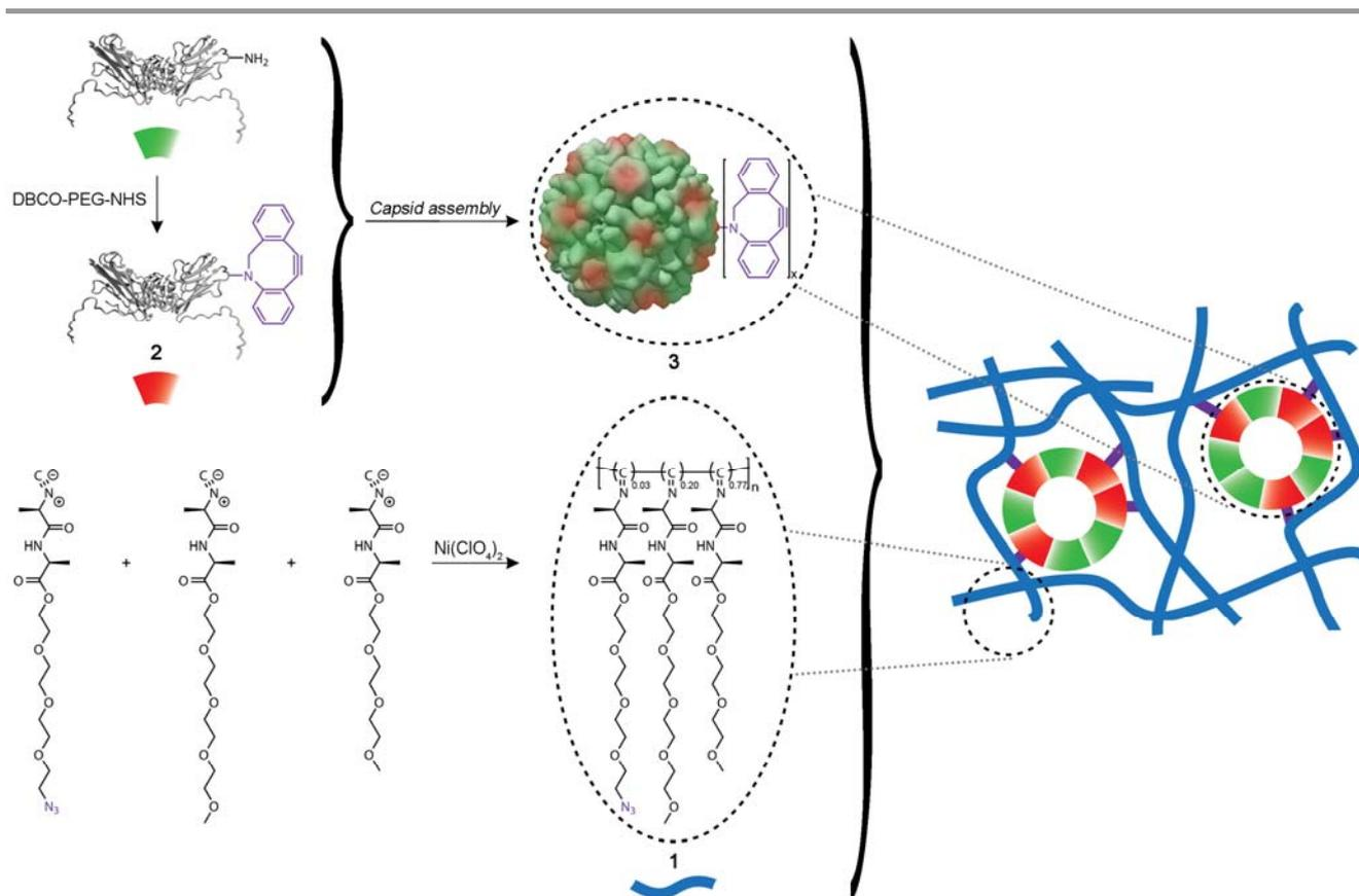
**Figure 1.** Schematic overview showing the crosslinking of an azide-functionalised polyisocyanide (PIC) hydrogel with DBCO-functionalised cowpea chlorotic mottle virus (CCMV) capsids. The PIC polymers **1** contain 3 % azide-functionalised monomers, 20 % tetra(ethylene glycol) monomers, and 77 % tri(ethylene glycol) monomers. The empty CCMV capsids **3** are assembled (pH change) from a mixture of capsid protein dimers with (red wedge, **2**) and without (green wedge) attached DBCO-groups.
