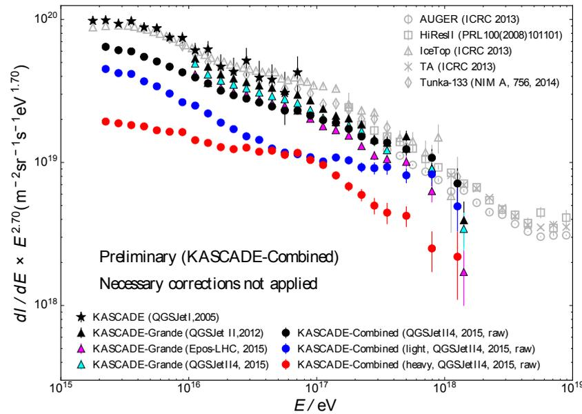
**Fig. 5.** The raw energy spectra of the all-particle (circles), light and heavy mass groups (blue and red circles, respectively) of cosmic rays reconstructed from the KASCADE-Grande combined analysis compared with the unfolded all-particle fluxes obtained with the KASCADE and KASCADE-Grande stand-alone analyses using QGSJET-II-02 (triangles) [24]. In the combined analysis the following post-LHC model QGSJET-II-04 was used for calibration purposes.
