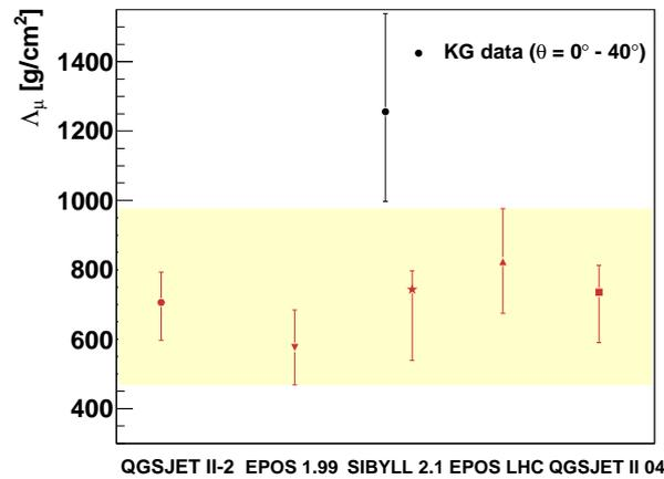
**Fig. 6.** Muon attenuation length of EAS data measured with the KASCADE-Grande experiment (upper point) compared with predictions of several pre-LHC and post-LHC high-energy hadronic interaction models (lower points) [26].
