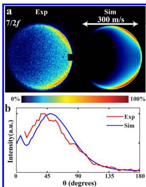
**Figure 5.** (a) Scattering image for the process  $\text{NO } (1/2f) + \text{He} \rightarrow \text{NO } (7/2f) + \text{He}$ , together with a simulated image based on the appropriate DCS predicted by theory. (b) Angular scattering distribution derived from the experimental and simulated images.
