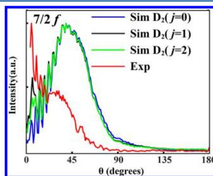
**Figure 7.** Experimental (Exp) and simulated (Sim) angular scattering distributions for  $\text{NO} + \text{normal-D}_2$  at a collision energy of  $720 \text{ cm}^{-1}$ , probing the final state  $(7/2f)$ . The simulations are performed assuming the hypothetical situation where the  $\text{D}_2$  molecules are exclusively in the  $j = 0$ ,  $j = 1$ , or  $j = 2$  rotational states.
