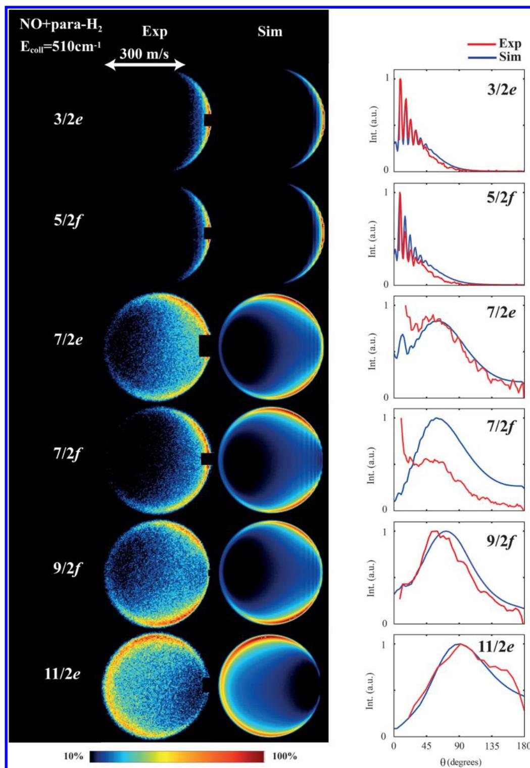
**Figure 3.** Scattering images for rotational inelastic collisions between NO ( $1/2f$ ) radicals and *para*-H<sub>2</sub> molecules, exciting the NO radicals to various final states. Left: Experimental (Exp) and simulated (Sim) ion images. Small segments of the images around forward scattering are masked because of the imperfect state selection of the NO packet. Right: Angular scattering distribution as derived from the experimental (red curves) and simulated (blue curves) images.
