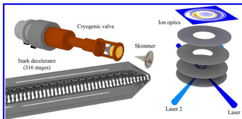
**Figure 1.** Schematic representation of the experimental setup. A beam of NO radicals is passed through a Stark decelerator and scattered with a pulsed beam of *para*-H<sub>2</sub> or *ortho*-D<sub>2</sub>. The inelastically scattered NO radicals are state-selectively ionized using two pulsed lasers and detected using velocity map imaging. Only the last section of the Stark decelerator is shown.
