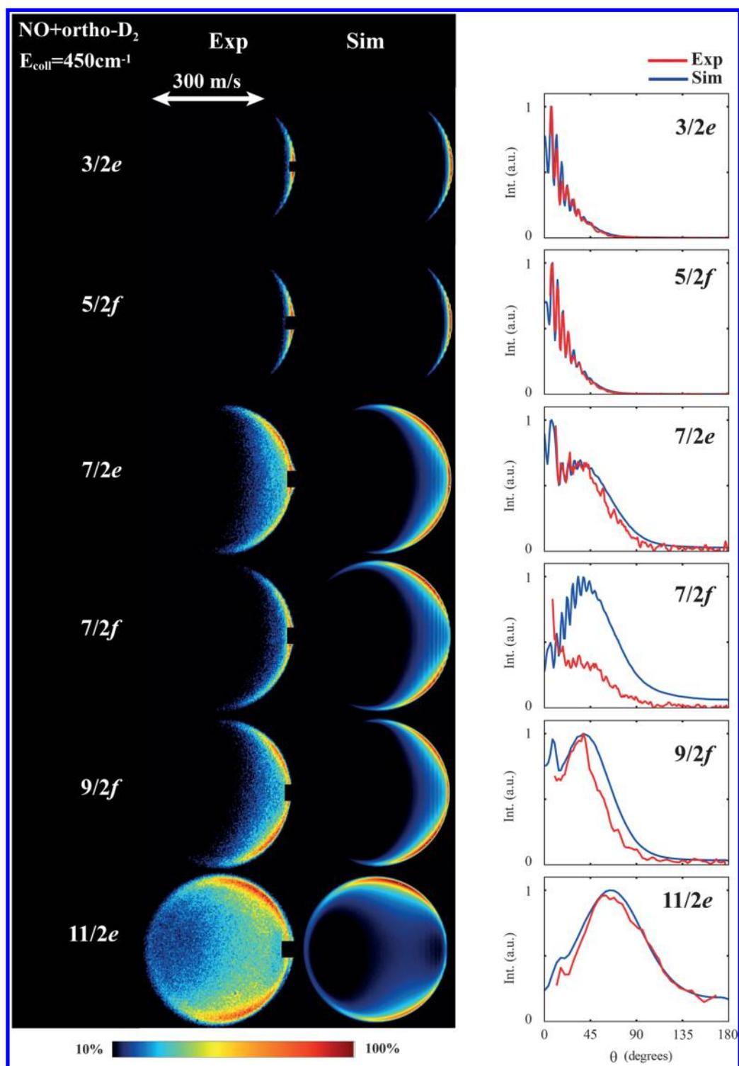
**Figure 4.** Scattering images for rotational inelastic collisions between NO ( $1/2f$ ) radicals and *ortho*-D<sub>2</sub> molecules, exciting the NO radicals to various final states. Left: Experimental (Exp) and simulated (Sim) ion images. Small segments of the images around forward scattering are masked because of the imperfect state selection of the NO packet. Right: Angular scattering distribution as derived from the experimental (red curves) and simulated (blue curves) images.
