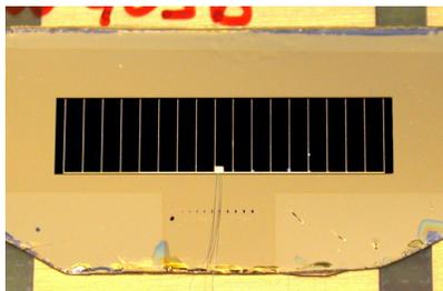
Figure 3: Photograph of a 1  $\text{cm}^2$  GaAs mirror cell.
