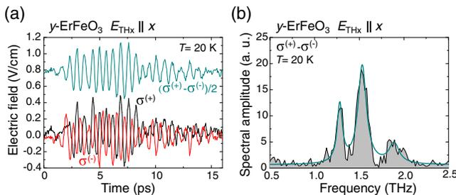
FIG. 4. (a) The THz waveforms generated in the y-cut  $\text{ErFeO}_3$  at 20 K by circularly polarized light of opposite helicities. The half-difference of these waveforms is shown shifted along the vertical axis. (b) The spectrum of the helicity dependent contribution obtained by Fourier transformation of the waveform shown in (a) and fitted with three Lorentzian contours.
