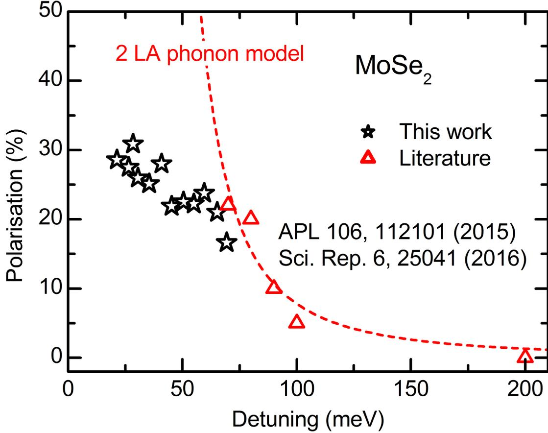
**Figure 6.** Measured degree of circular polarization of PL emission from MoSe<sub>2</sub> as a function of detuning between excitation and exciton transition energy. Values at large detuning (triangles) are taken from the literature [30, 33]. The dashed line is calculated dependence for two LA phonon model using  $\hbar\omega_{2LA} = 38$  meV and  $\alpha = 0.1$ .
