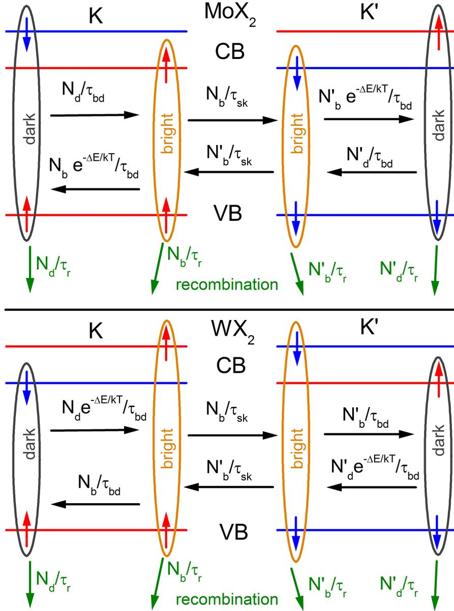
**Figure 1.** Schematic showing the band structure and spin configuration of the bright and dark A-excitons in MoX<sub>2</sub> and WX<sub>2</sub> materials. The possible inter and intra valley scattering and recombination paths included in the rate equations (see text) are indicated schematically. The influence of B-excitons can safely be neglected due to the large spin-orbit splitting in the valence band.
